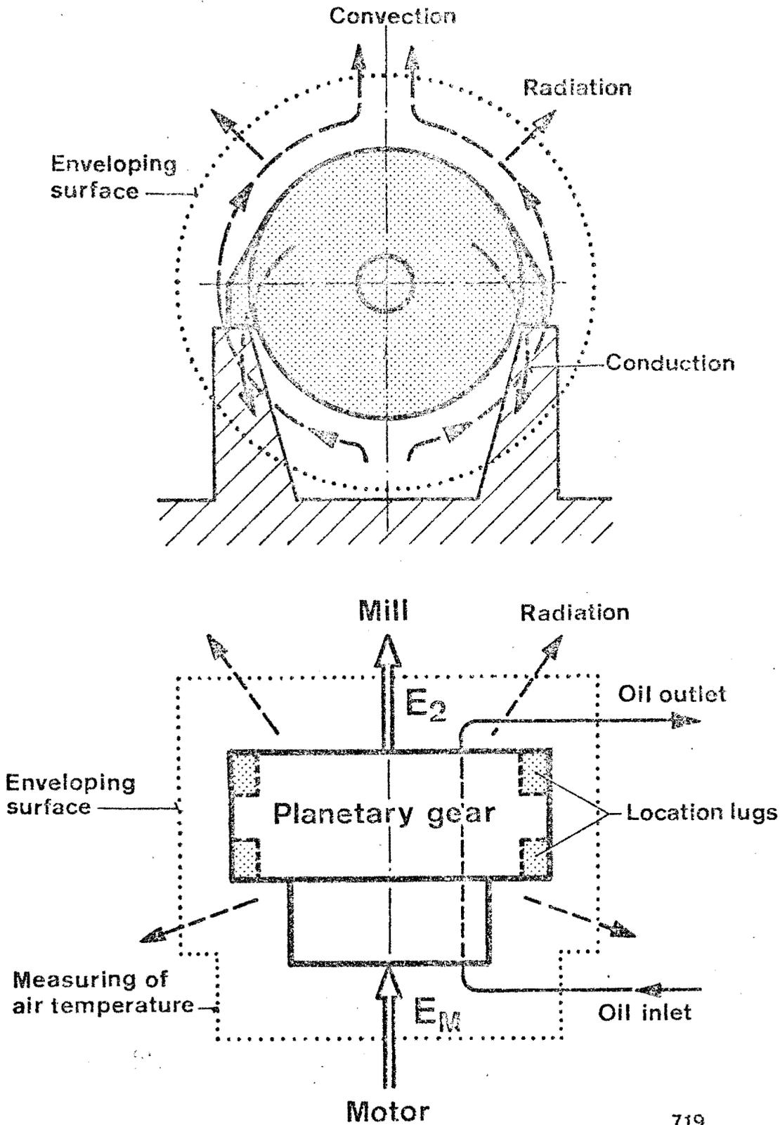
Fig. 2 Measuring principle. Heat dissipation losses via convection, radiation and conduction.
